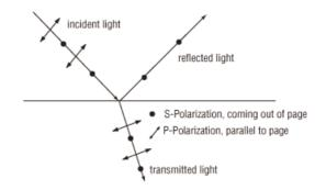
When referring to polarization states, the p-polarization refers to the polarization plane parallel to the polarization axis of the polarizer being used ("p" is for "parallel"). The s-polarization refers to the polarization plane perpendicular to the polarization axis of the polarizer. A linear polarizer, by design, polarizes light in the p-polarization.
